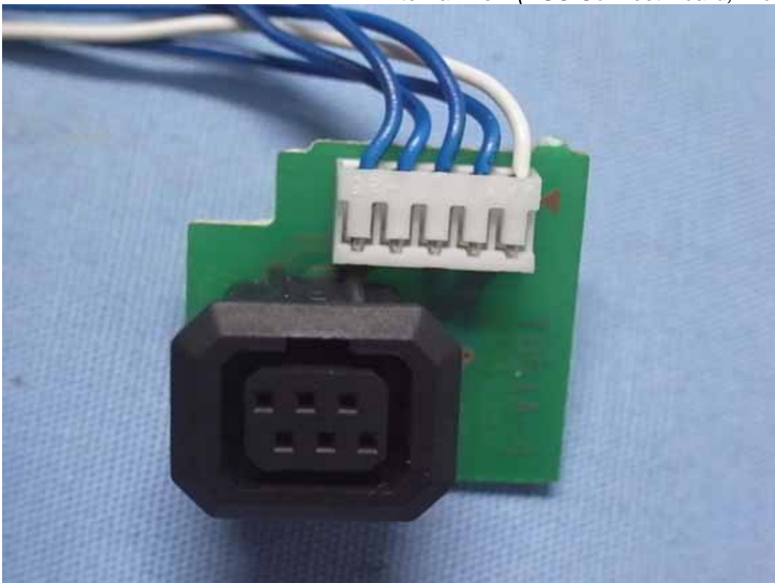
Figure 16 Internal View (DSC Connect Board, Front View)
