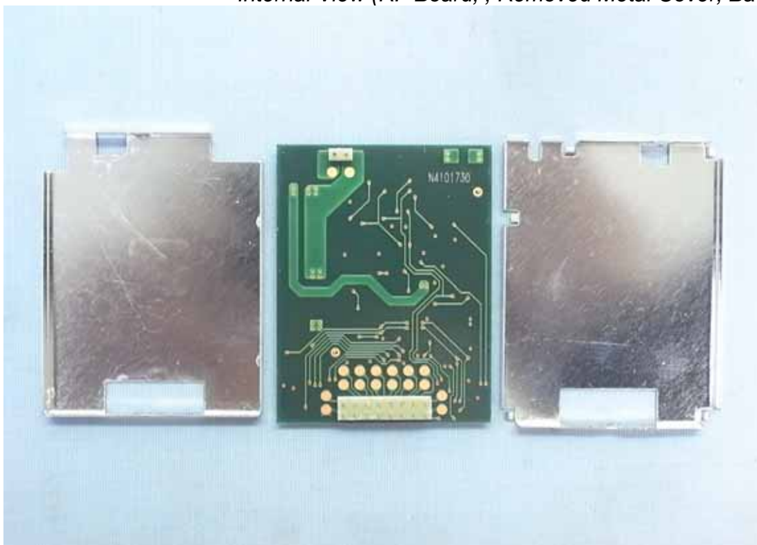
Figure 24 Internal View (RF Board, , Removed Metal Cover, Back View)
