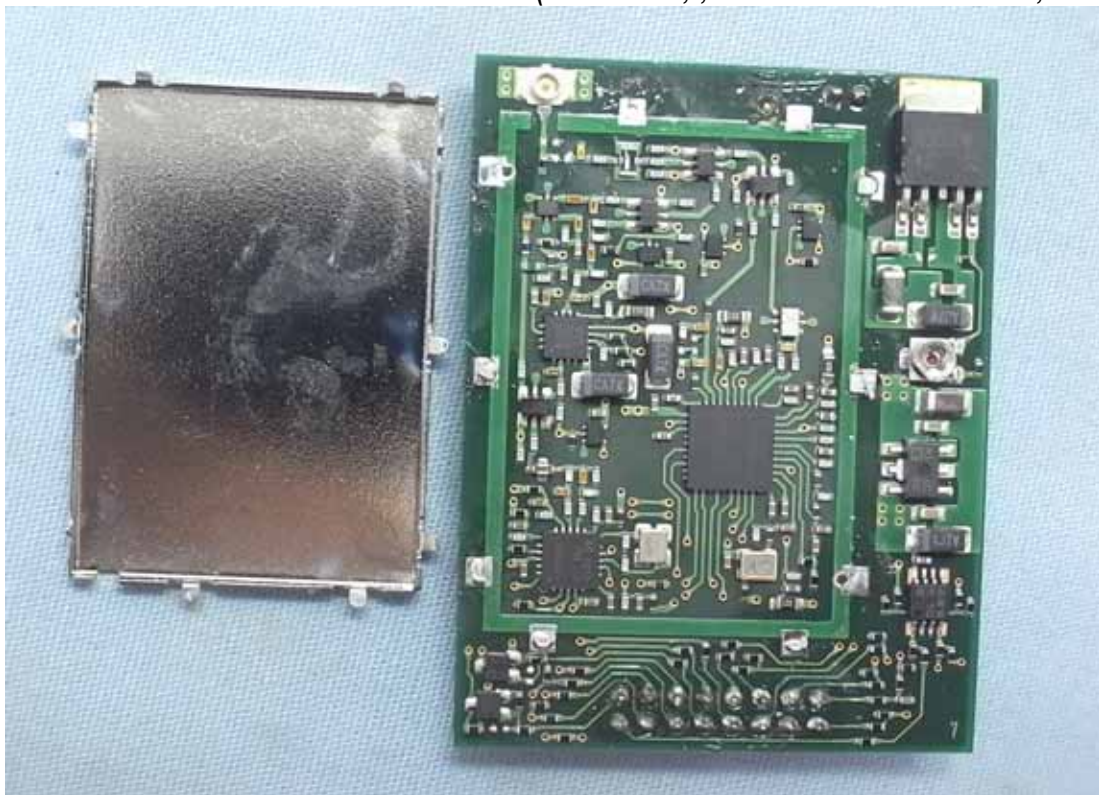
Figure 23 Internal View (RF Board, , Removed Metal Cover, Front View)
