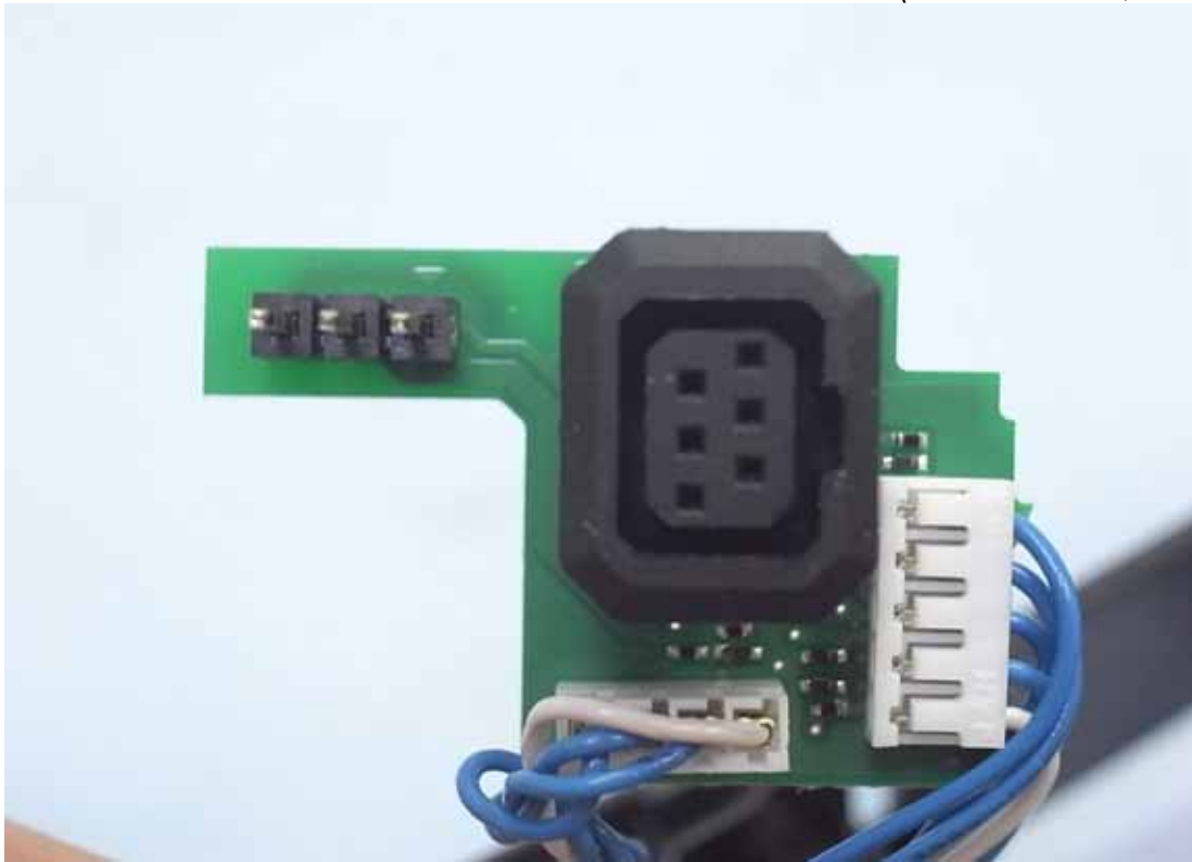
Figure 17 Internal View (Control Board, Front View)
