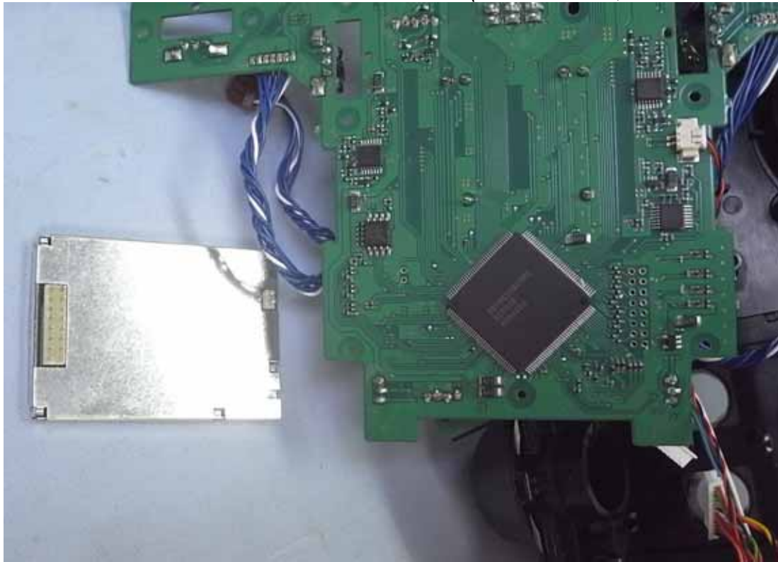
Figure 21 Internal View (Control Board, Removed Metal Cover)
