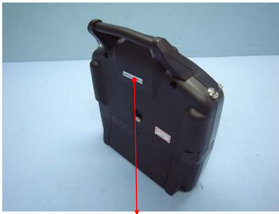
FCC Label Placement Location
