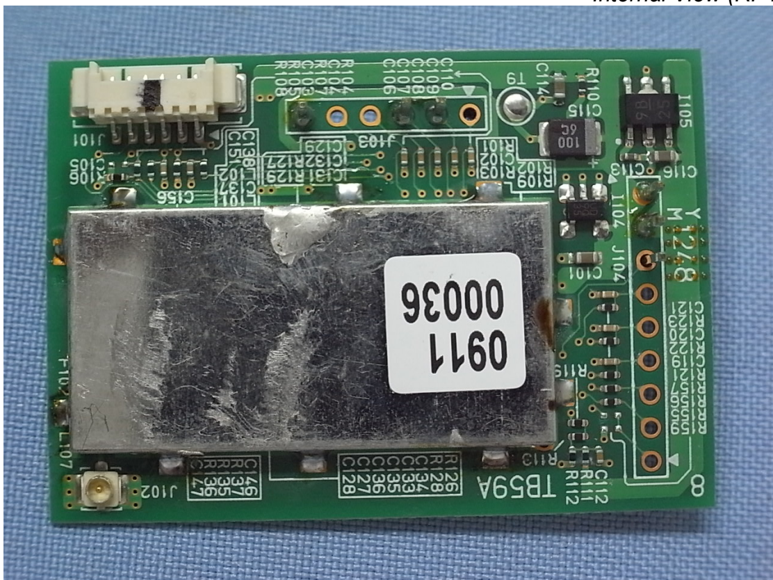
Figure 6 Internal View (RF Module)
