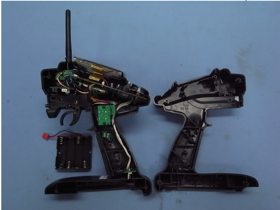
Figure 5 Internal View (Removed Cover)
