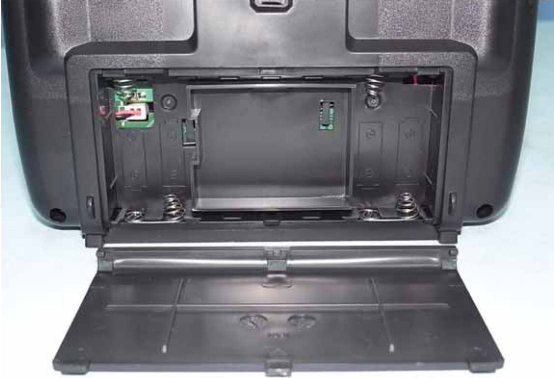
Figure 5 Internal View (Removed Battery Cover)
