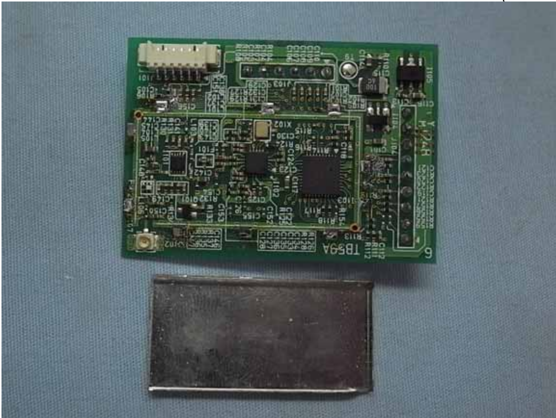
Figure 9 Internal View (RF Board)
