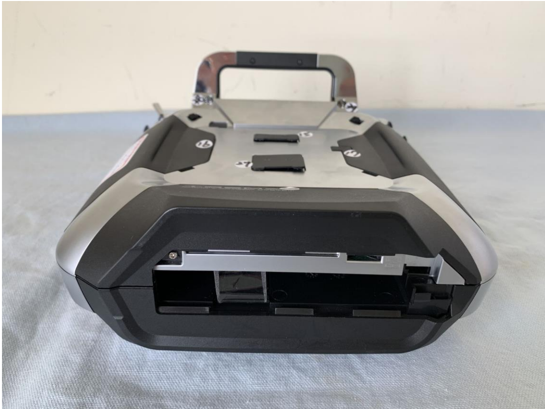
Figure 12 Internal View (Removed Battery Cover)
