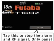
and RF signal. Only panel screen operation is active, the transmitter will not link to any receiver.
