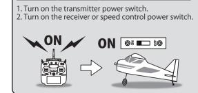
Turning on the power switches
