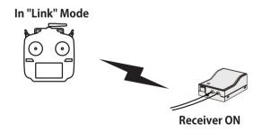
8. If linking fails, an error message is displayed. Bring the transmitter closer to the receiver and repeat the procedure above from Step 2.
