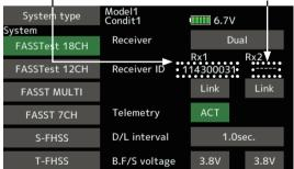
In Dual, a primary receiver (Rx1) is linked first. Next, a secondary (Rx2) receiver is linked.
