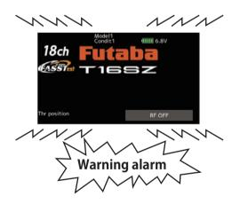
When the alarm activates, lower the throttle stick before turning the receiver power ON.
