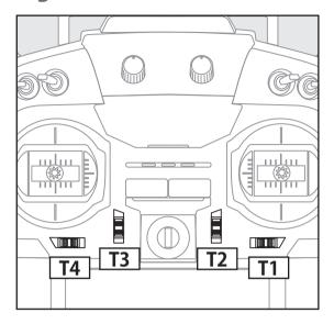
This transmitter is equipped with 4 digital trims. Each time you press a trim button, the trim position moves one step. If you continue pressing it, the trim position starts to move faster. In addition, when the trim position returns to the center, the tone will change. You can always monitor trim positions by referencing the LCD screen.
