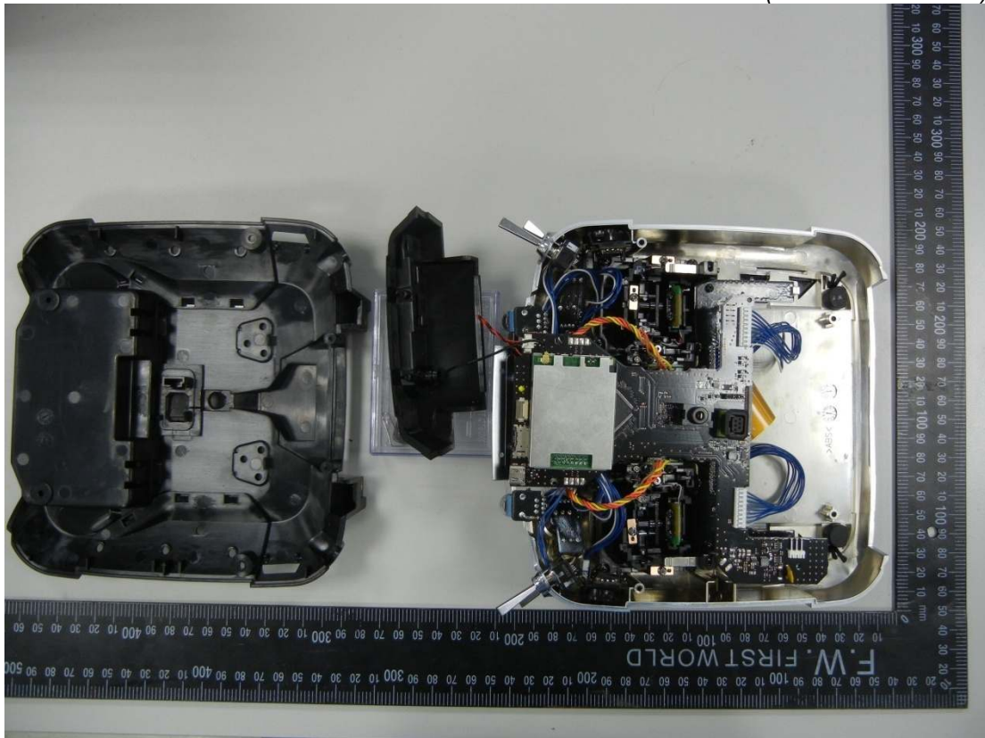
Figure 16 Internal View (Removed Cover)
