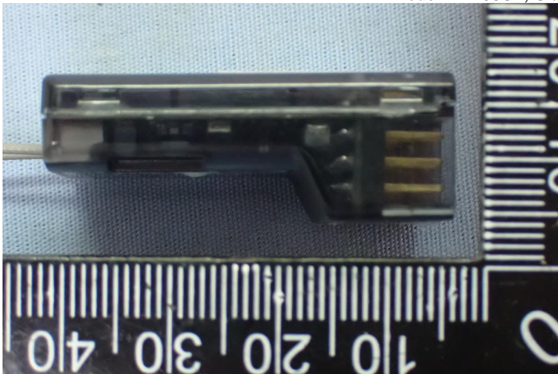
Figure 12 General Appearance with Antenna Ant 2-Gray (UFL-LP6-068N1T-A11-T-153D) Model: R7208SB, Side View
