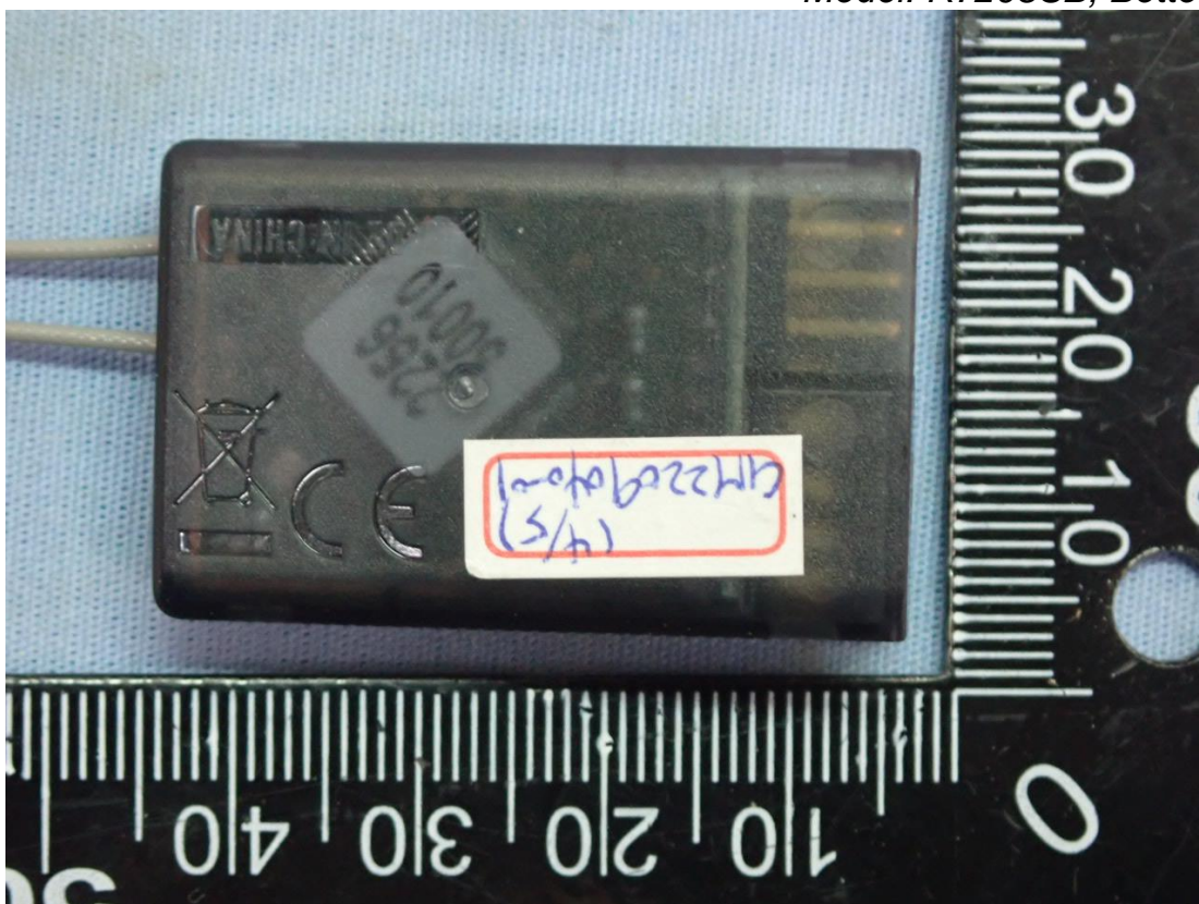
Figure 10 General Appearance with Antenna Ant 2-Gray (UFL-LP6-068N1T-A11-T-153D) Model: R7208SB, Bottom View
