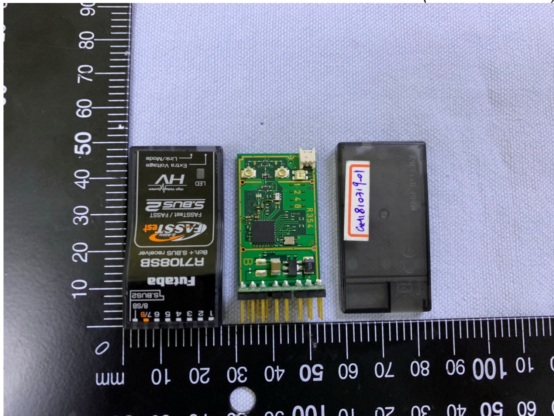
Figure 7 Internal View (Removed Covers)
