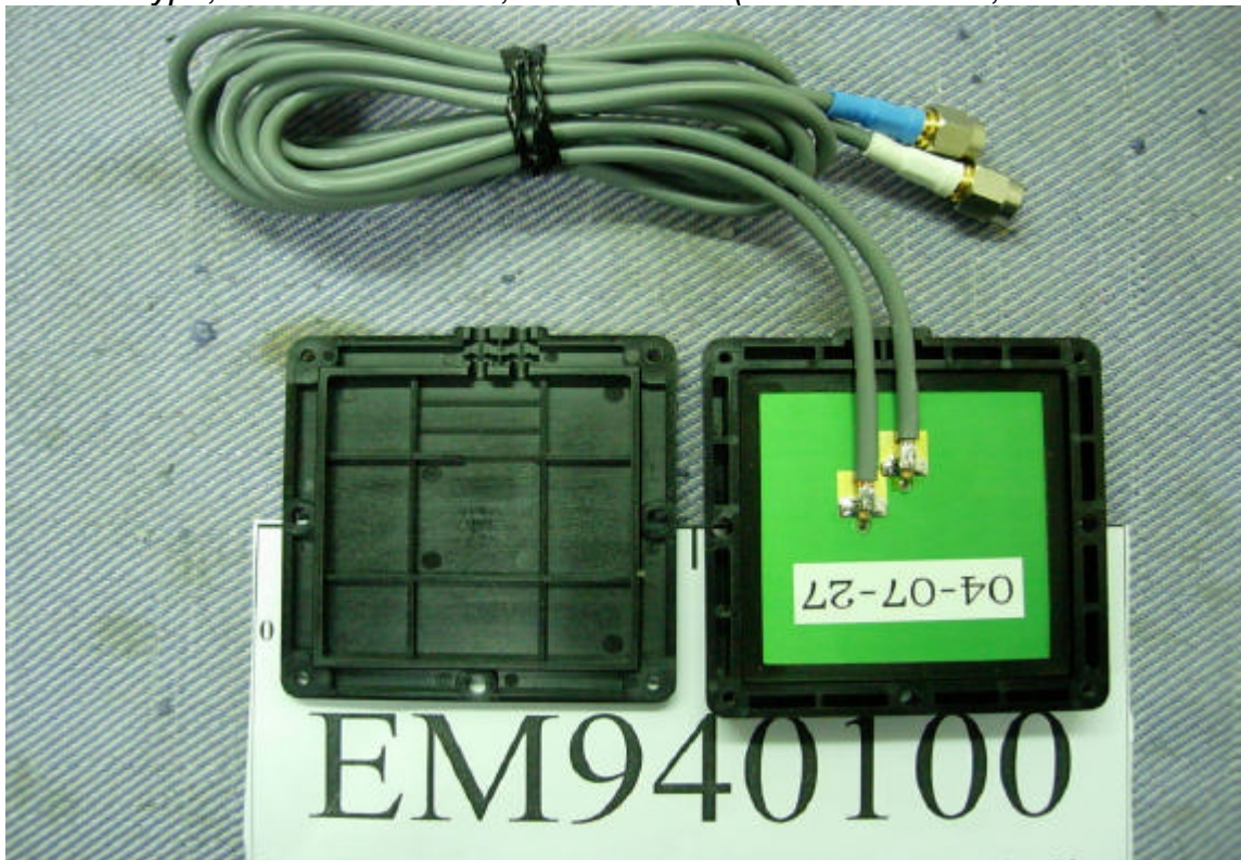
Flat Type, Two CoAx Cables, Internal View (Removed Cover, Antenna/Back View)
