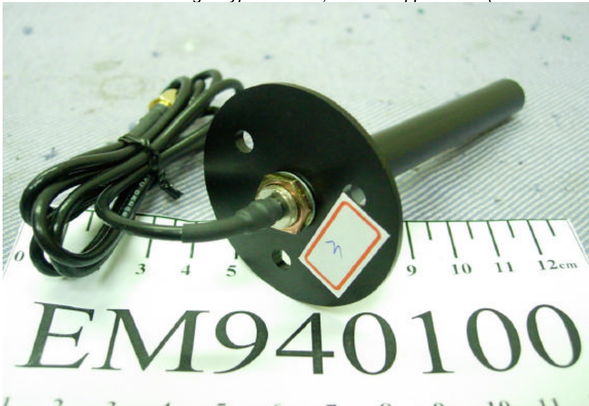
Figure 10 Pedestal Base with Rigid Type Antenna, General Appearance (Back & Side View)
