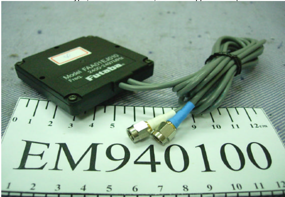
Figure 12 Flat Type, Two CoAx Cables, General Appearance (Back & Side View)
