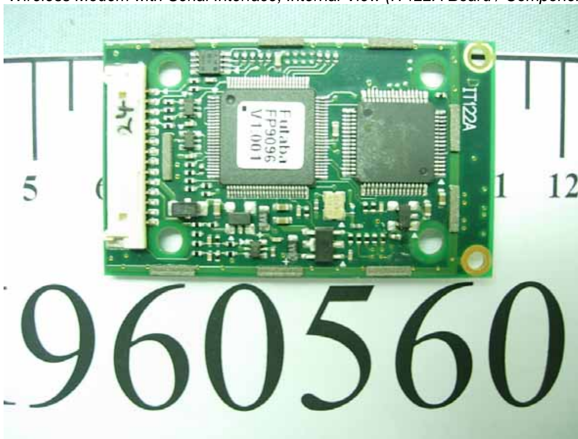
Wireless Modem with Serial Interface, Internal View (IT122A Board / Component Side)
