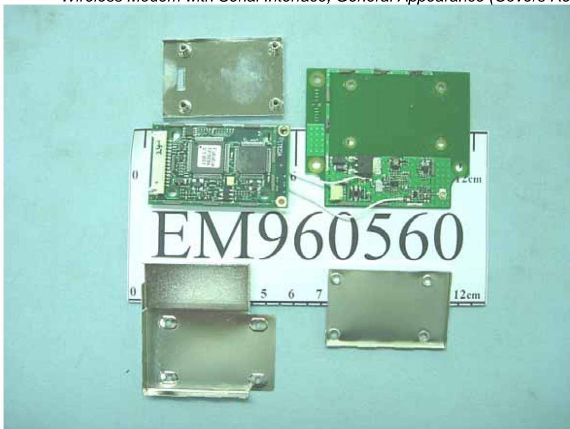
Figure 3 Wireless Modem with Serial Interface, General Appearance (Covers Removed)
