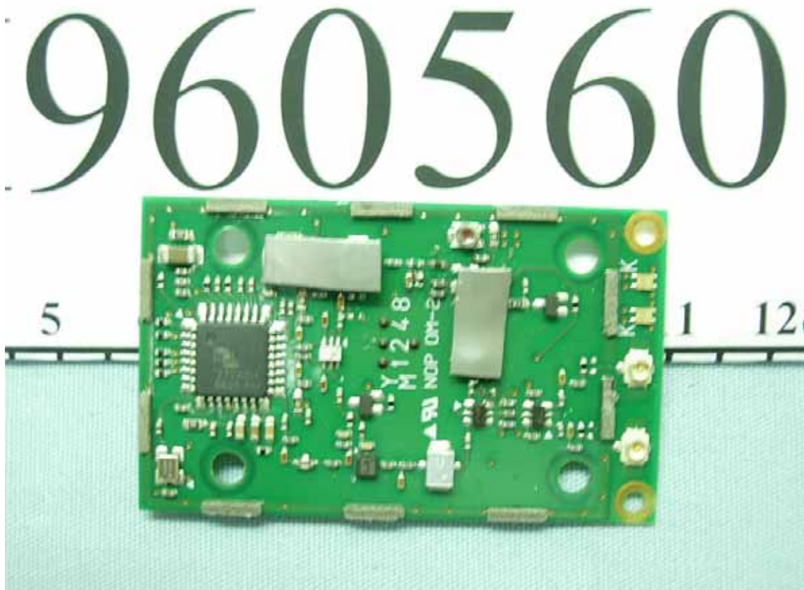
Figure 7 Wireless Modem with Serial Interface, Internal View (IT122A Board / Foil Side)
