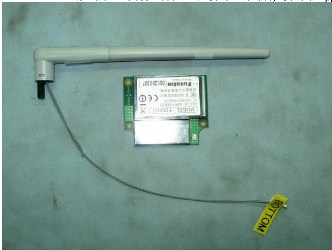
Figure 10 Antenna & Wireless Modem with Serial Interface, General Appearance
