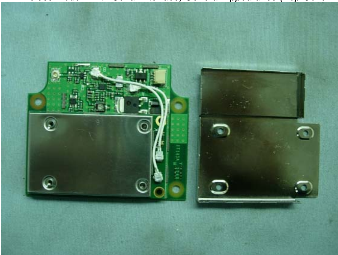
Figure 3 Wireless Modem with Serial Interface, General Appearance (Top Cover Removed)
