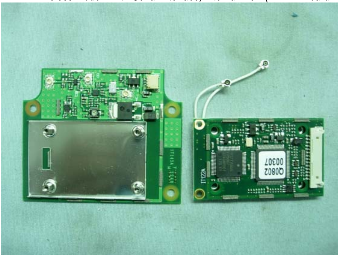
Figure 4 Wireless Modem with Serial Interface, Internal View (iT122A Board Removed)
