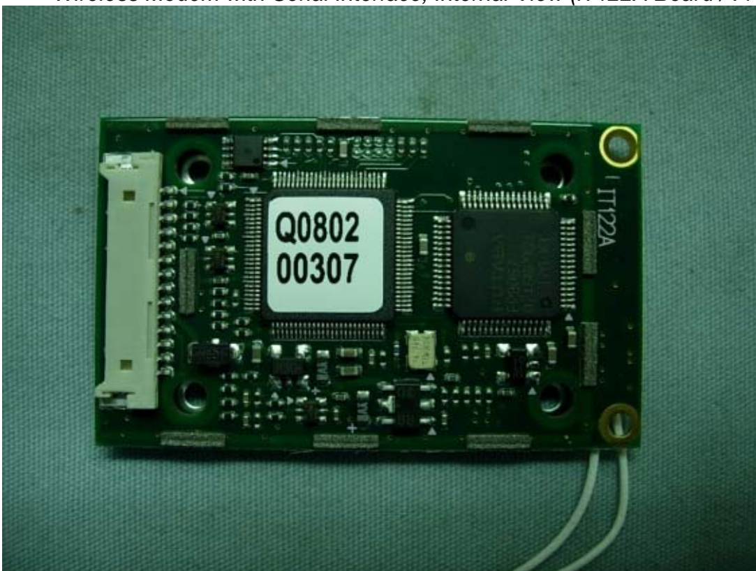
Wireless Modem with Serial Interface, Internal View (iT122A Board / Front View)
