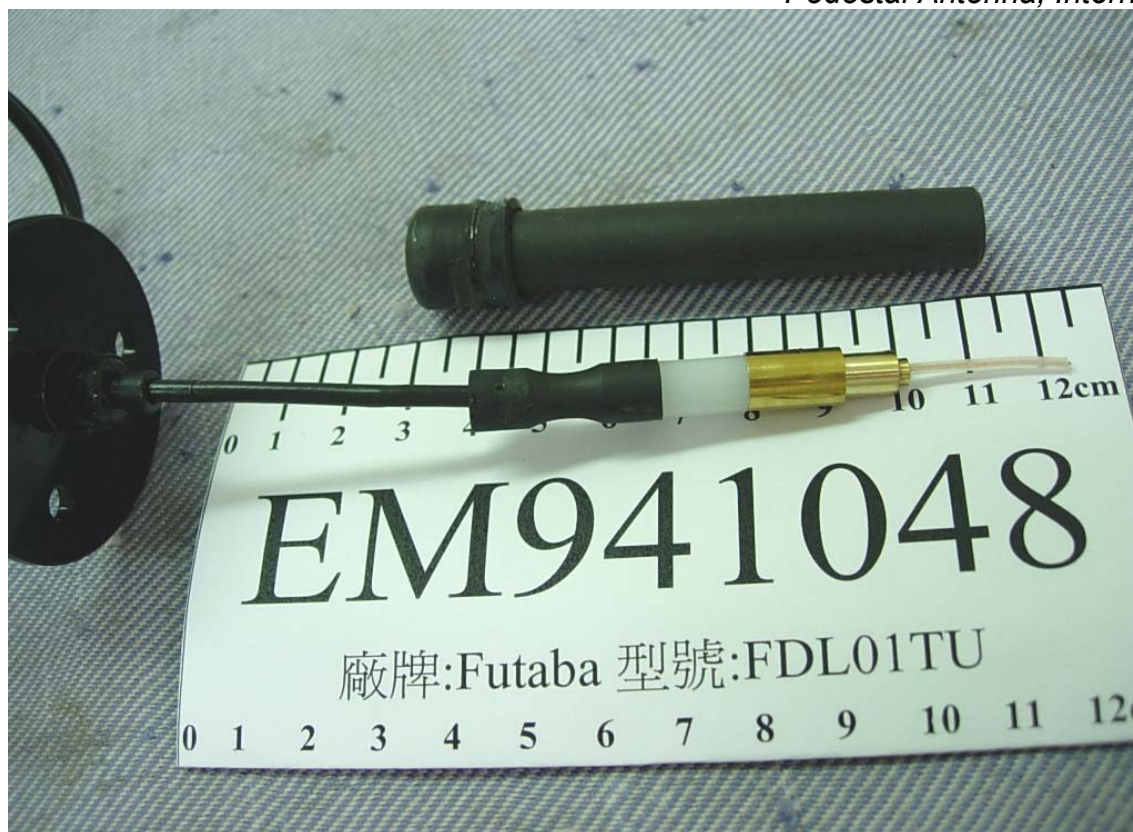
Figure 13 Pedestal Antenna, Internal View
