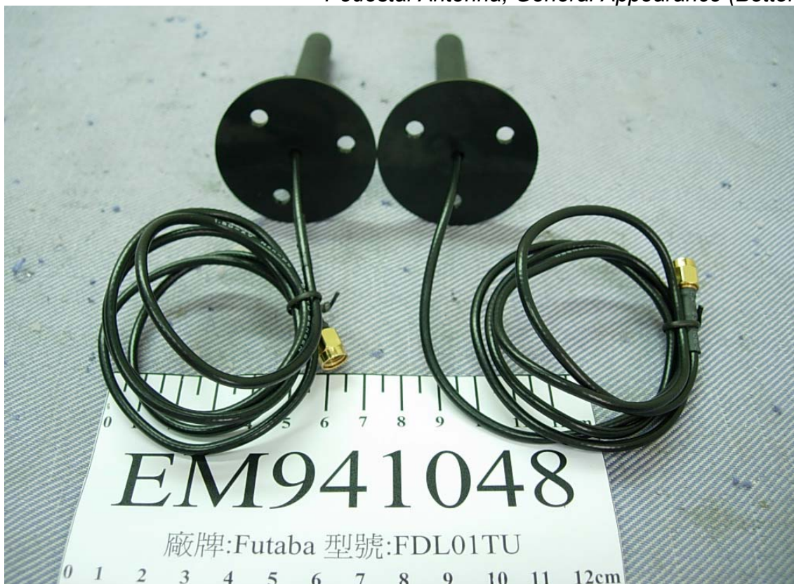
Figure 12 Pedestal Antenna, General Appearance (Bottom View)
