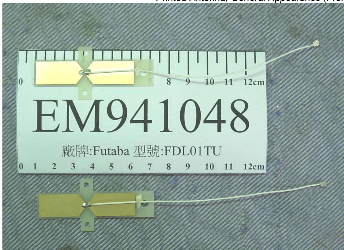
Figure 7 Printed Antenna, General Appearance (Front View)
