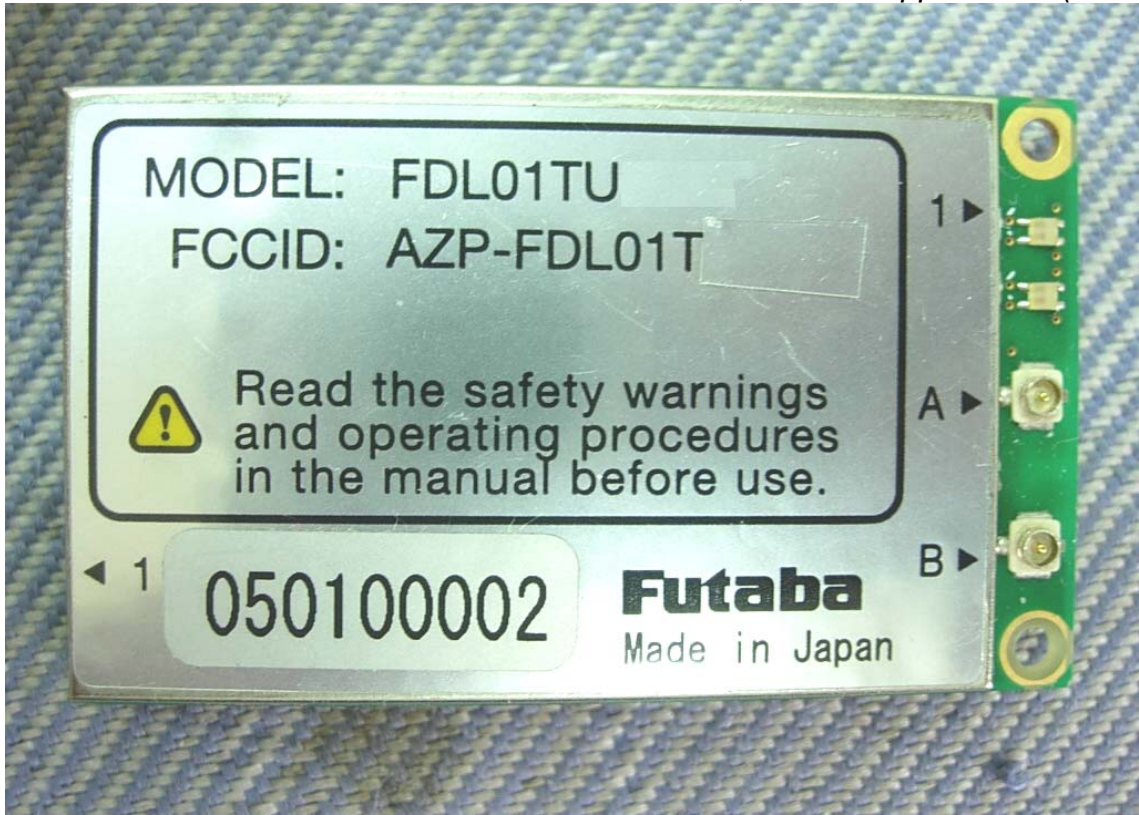
Wireless Modem with Serial Interface, General Appearance (Front View)
