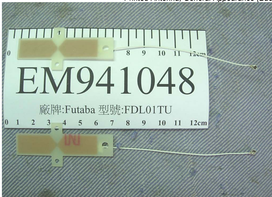
Figure 8 Printed Antenna, General Appearance (Back View)
