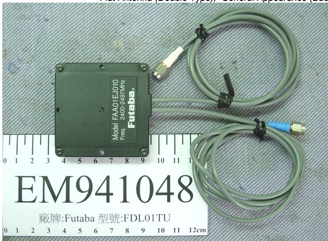
Figure 19 Flat Antenna (Double Type), General Appearance (Back View)
