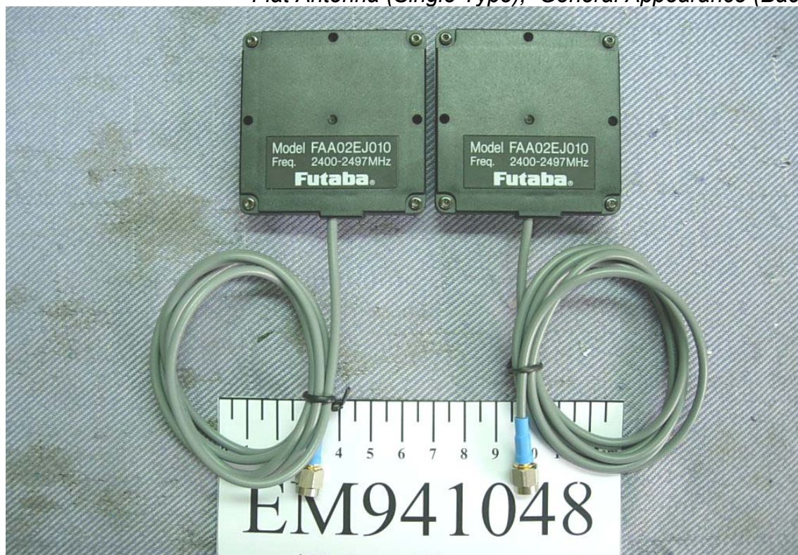
Figure 15 Flat Antenna (Single Type), General Appearance (Back View)
