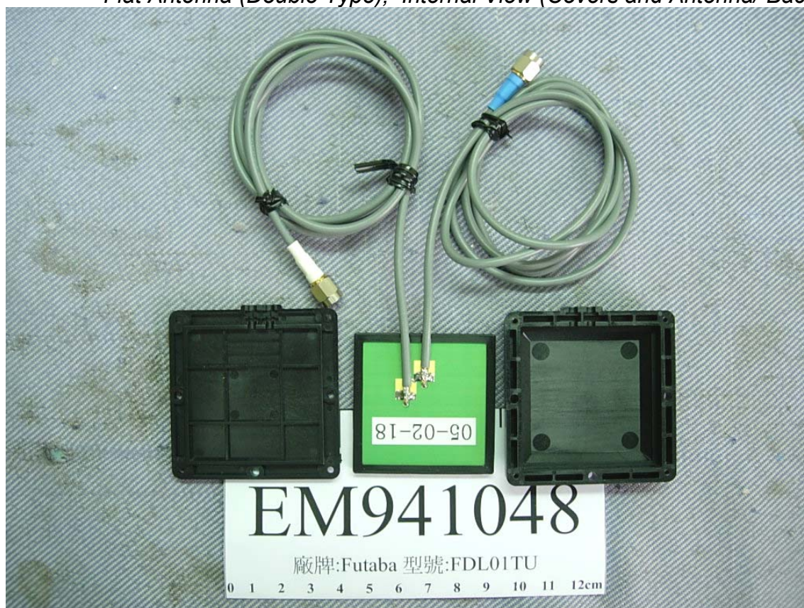
Figure 20 Flat Antenna (Double Type), Internal View (Covers and Antenna/ Back View)
