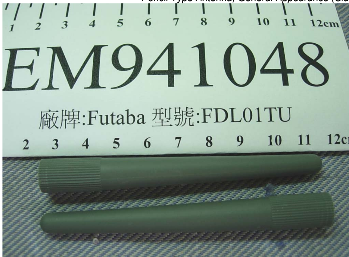
Figure 10 Pencil Type Antenna, General Appearance (Side View)
