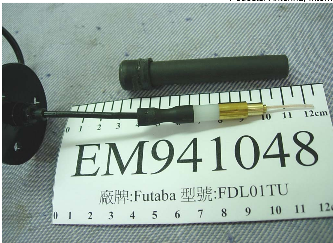
Figure 13 Pedestal Antenna, Internal View
