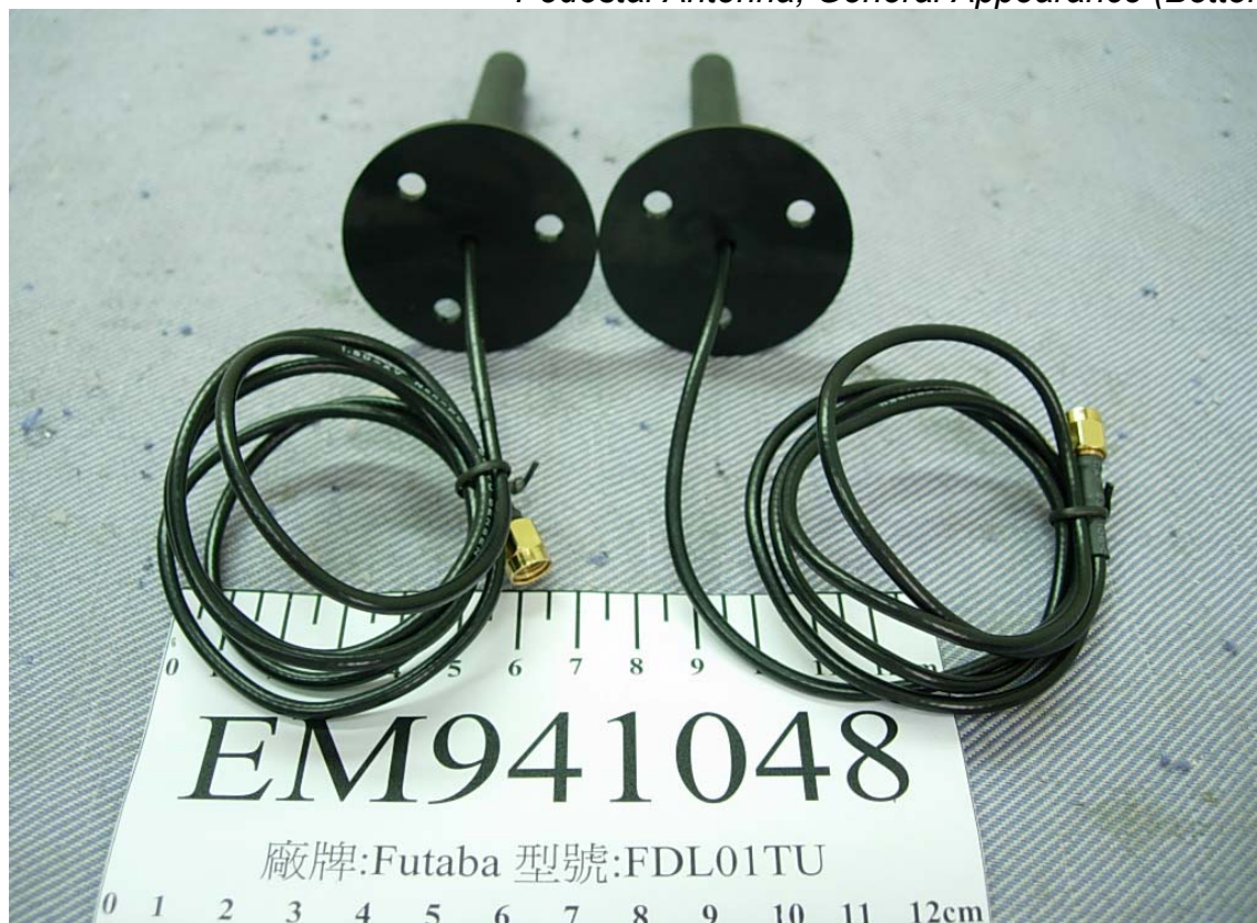
Figure 12 Pedestal Antenna, General Appearance (Bottom View)
