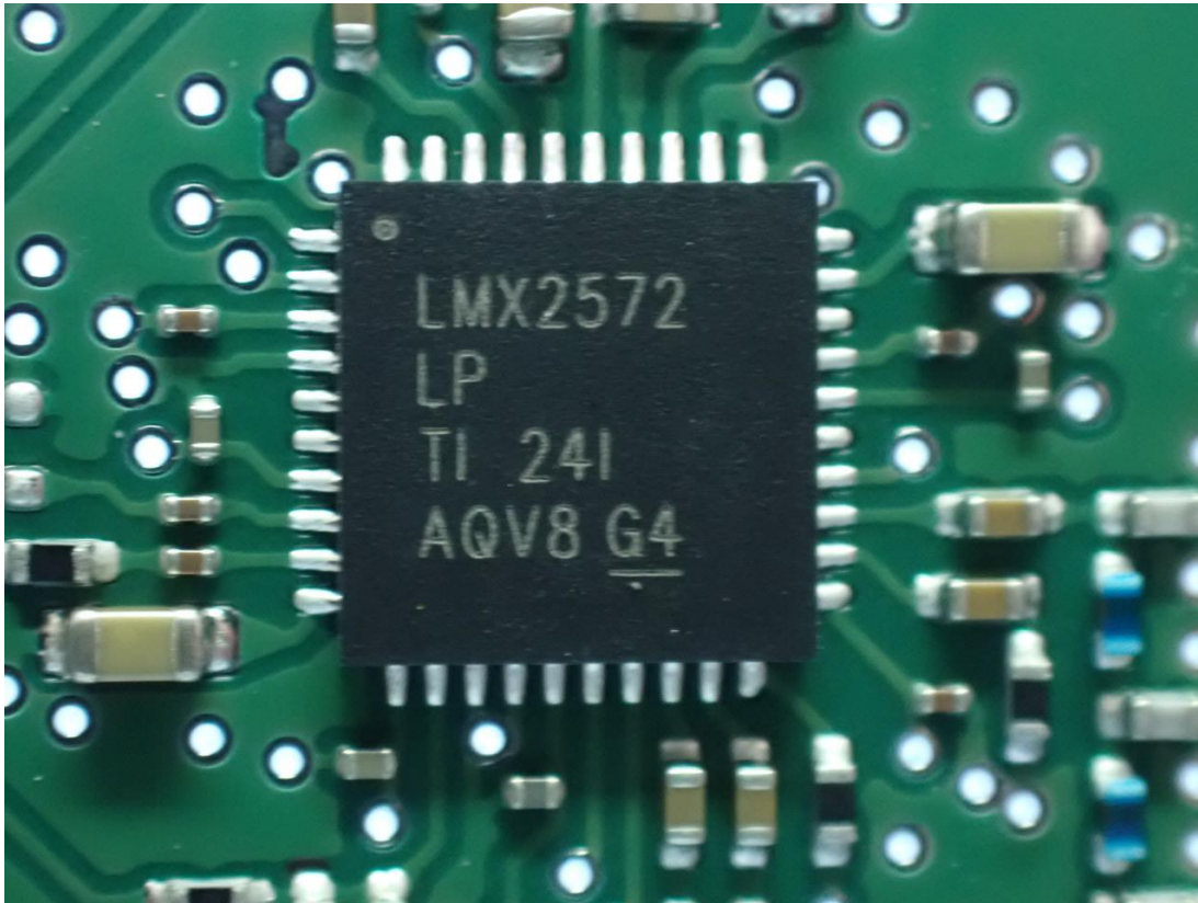
Figure 27 RF IC#1: LMX2572
