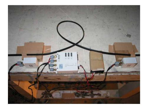
8.2a Setup with the Maximized RFI Field Strength Emission Level (Open Field Test Site No.1)
