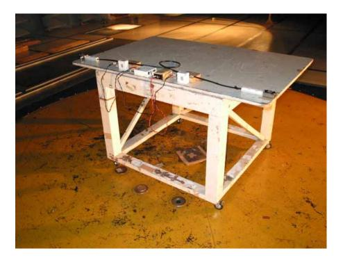
8.1b Setup with the Maximized RFI Field Strength Emission Level (Semi Anechoic Chamber)
