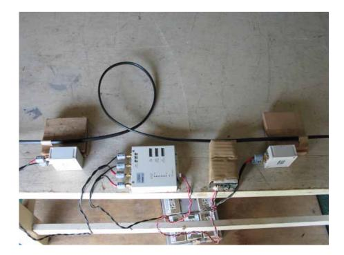
8.3a Setup with the Maximized RFI Field Strength Emission Level (Open Field Test Site No.6)
