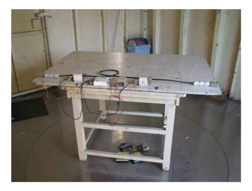
8.3b Setup with the Maximized RFI Field Strength Emission Level (Open Field Test Site No.6)
