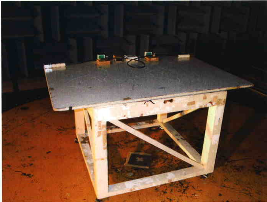
Photo 7.1a Setup with the Maximized RFI Field Strength Emission Level (Semi Anechoic Chamber)
