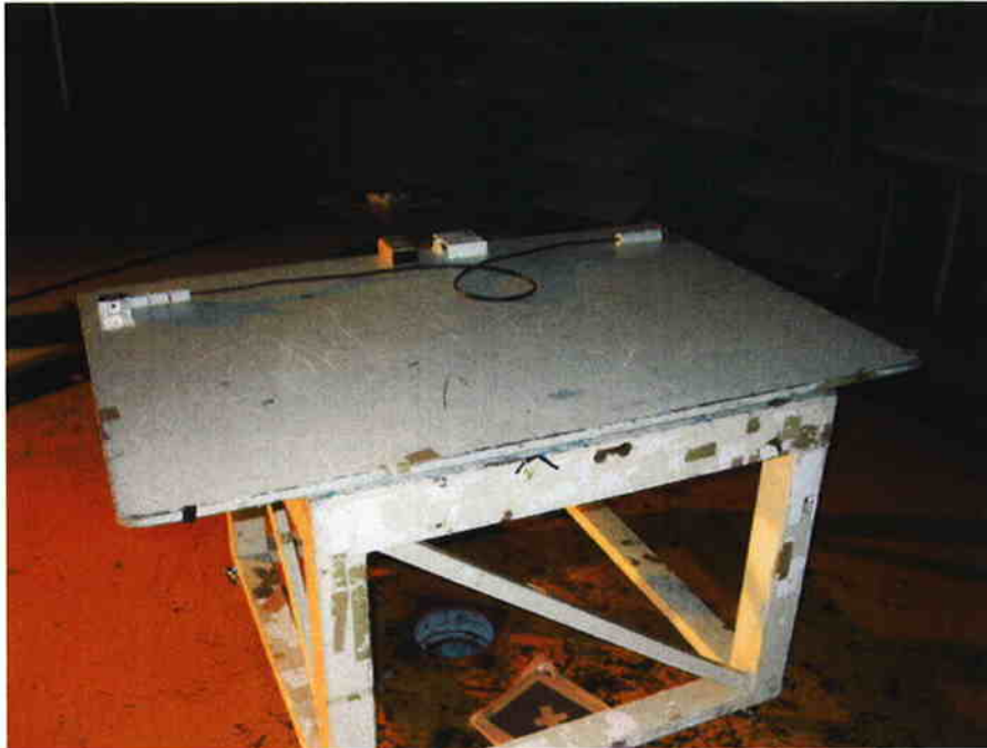
Photo 7.1a Setup with the Maximized RFI Field Strength Emission Level
