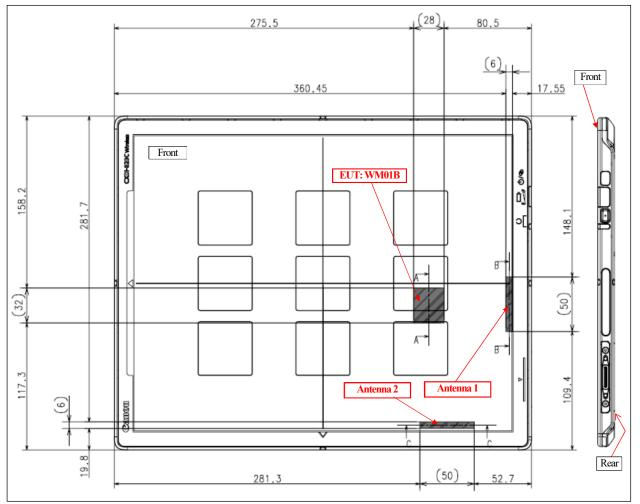
\*. Size of host platform: 308 × 384 × 15.5 (thickness) [mm] (\*. Size of EUT: 28 (W) × 32 (D) × 3 (thickness) [mm])
