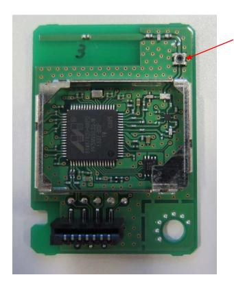
This antenna connector is used for inspection only.
