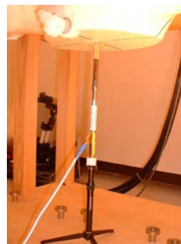
2450MHz System performance check setup
