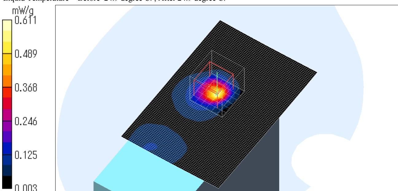
**3.Measurement data (Head SAR 2450MHz)**
