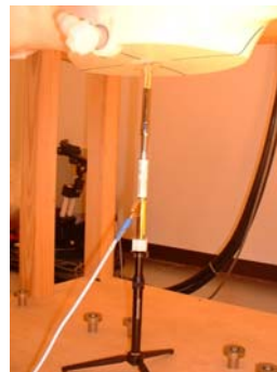
2450MHz System performance check setup
