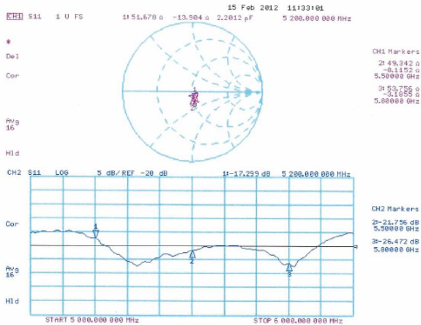
**Impedance Measurement Plot for Head TSL (UL Spacer #2)**
