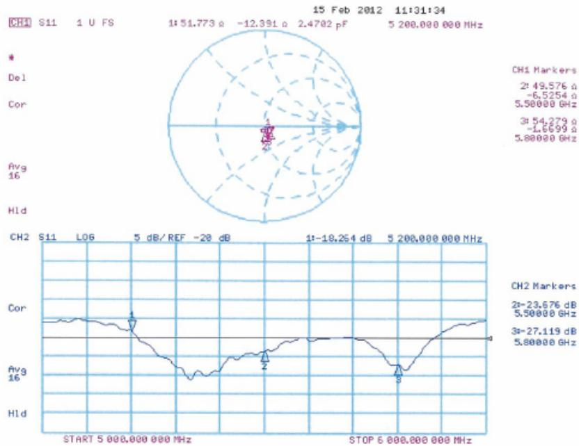
**Impedance Measurement Plot for Body TSL (UL Spacer #2)**
