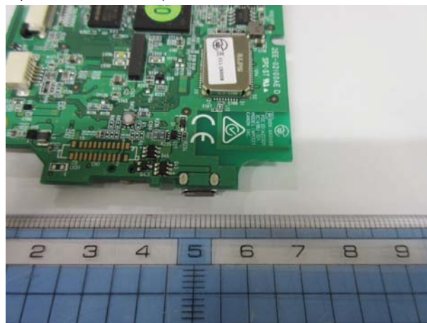
MAIN PCB (WLAN MODULE) – RF Part and Antenna –
