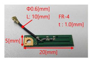
Antenna with GND plate for tests
