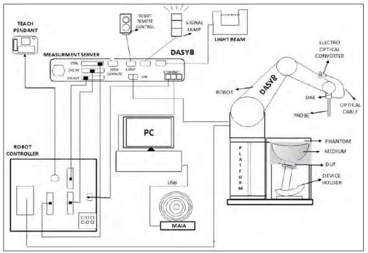
The DASY8 SAR/APD system for performing compliance tests consist of the following items:
