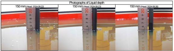
Dipole: D5GHzV2-1070-2401 ; Mode: CW(0) ; Frequency: 5250.000 MHz ; Test Distance: 10 mm (dipole to liquid); Power setting: 17.0 dBm TSL parameters used: Head(v6) ; f= 5250.000 MHz; Conductivity: 4.528 S/m; Permittivity: 34.62
