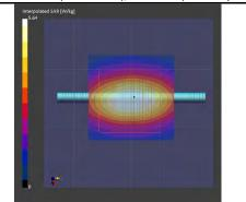
Remarks: \*. Date tested:2024-08-26 ; Tested by: Akihiro Oda; Tested place:No.7 shielded room; Ambient: 24 deg.C. / 45 %RH; Liquid depth: 150 mm; \*. Liquid temperature: 22.5 deg.C. ± 0.5 deg.C. (22.5 deg.C., in check); \*. Red cubic: big=SAR(10g ) / small=SAR(1) \*. Project file name-Measurement Group: 240822\_15407507\_es204(7)+ds126907.d8sar- SPC Measurement Group:
