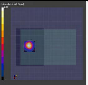
\*. Date tested: 2024-08-22;Tested by: Akihiro Oda; Tested place:No.7 shielded room; Ambient: 24 deg.C. / 61 %RH; Liquid depth: 150 mm; \*. Liquid temperature: 22.5 deg.C. ± 0.5 deg.C. (22.5 deg.C., in check); \*. Red cubic: big=SAR(10g ) / small=SAR(1g) \*. Project file name-Measurement Group: 240822\_15407507\_es204(7)+ds126907.d8sar- 8/22-5,11a,5300,front-left Remarks:
