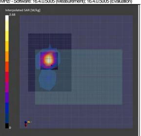
Remarks: \*. Date tested: 2024-08-22;Tested by: Akihiro Oda; Tested place:No.7 shielded room; Ambient: 22 deg.C. / 78 %RH; Liquid depth: 150 mm; \*. Liquid temperature: 22.5 deg.C. ± 0.5 deg.C. (22.5 deg.C., in check); \*. Red cubic: big=SAR(10g) / small=SAR(10) \*. Project file name-Measurement Group: 240822\_15407507\_es204(7)+ds126907.d8sar- 8/22-1,11a,5240,front-left
