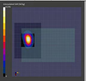
Remarks: \*. Date tested: 2024-08-26;Tested by: Akihiro Oda; Tested place:No.7 shielded room; Ambient: 24 deg.C. / 54 %RH; Liquid depth: 150 mm; \*. Liquid temperature: 22.5 deg.C. ± 0.5 deg.C. (22.5 deg.C., in check); \*. Red cubic: big=SAR(10g ) / small=SAR(10) \*. Project file name-Measurement Group: 240822\_15407507\_es204(7)+ds126907.d8sar- 8/26-3,11b,2462,front-left
