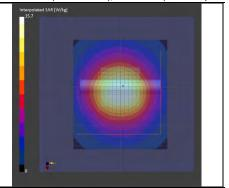
Remarks: \*. Date tested:2024-08-22; Tested by: Akihiro Oda; Tested place:No.7 shielded room; Ambient: 22.4 deg.C. / 64 %RH; Liquid depth: 150 mm; \*. Liquid temperature: 22.5 deg.C. ± 0.5 deg.C. (22.5 deg.C., in check); \*. Red cubic: big=SAR(10g) / small=SAR(1); \*. Project file name-Measurement Group: 240822\_15407507\_es204(7)+ds126907.d8sar- SPC Measurement Group
