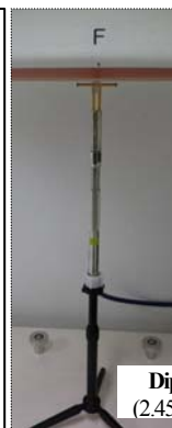
Test setup for the system performance check
