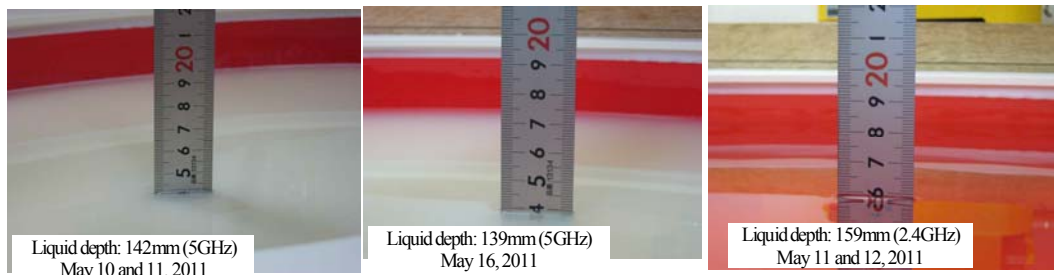
Test setup for the system performance check
