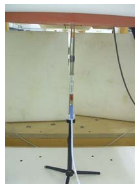
2450MHz System performance check setup
