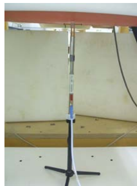
2450MHz System performance check setup
