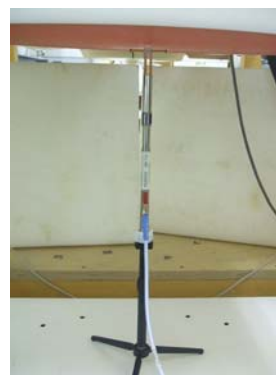
2450MHz System performance check setup
