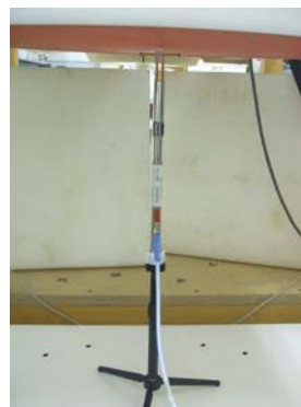
2450MHz System performance check setup
