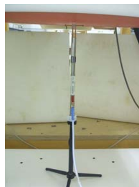
2450MHz System performance check setup
