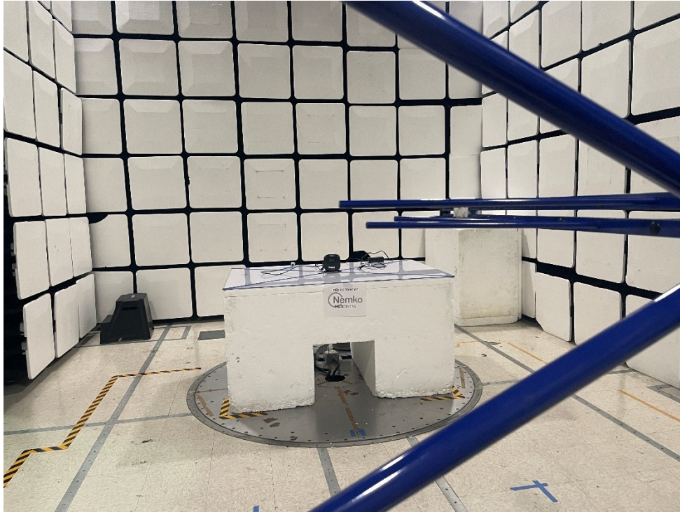
Figure 2 - Radiated emissions below 1 GHz (0.03 – 1 GHz), front view.
