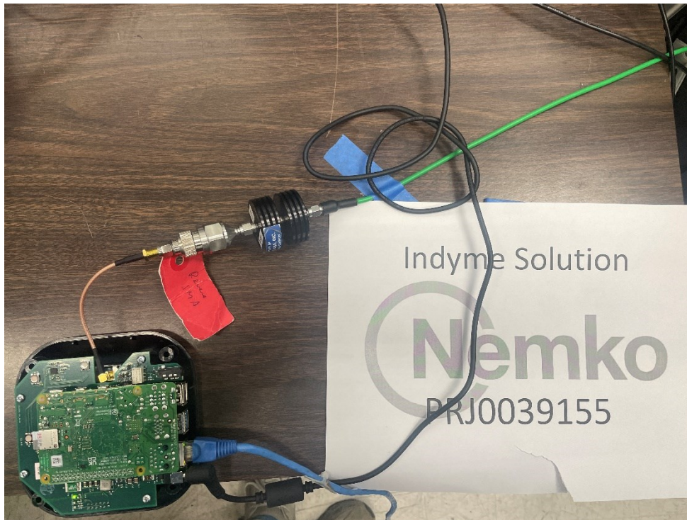
Figure 10 – Test setup: antenna conducted port.
