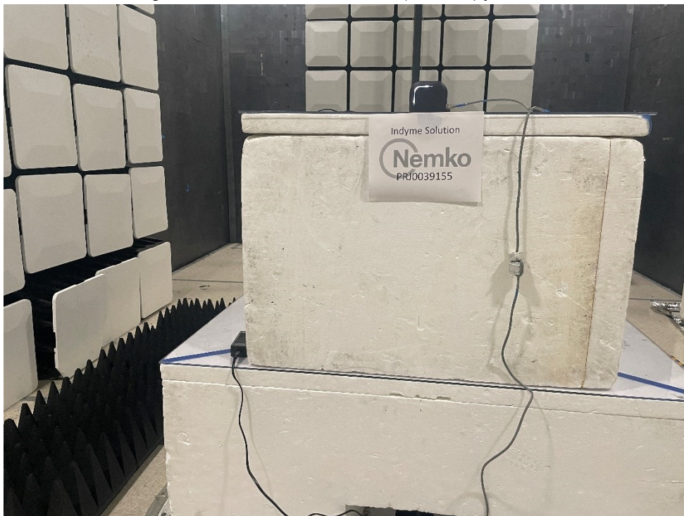
Figure 5 - Radiated emissions above 1 GHz (1 – 18 GHz), rear view.
