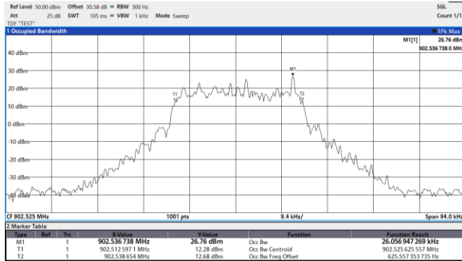
Figure 8.10-1: 99% occupied bandwidth, 902.525 MHz
