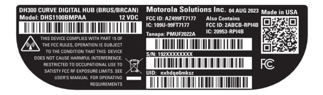
Figure 1: FCC/IC Label for DHS1100BMPAA
