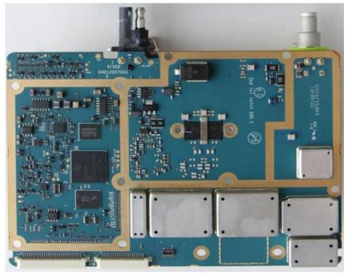
RF board with Shields (Bottom)
