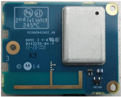
**Expansion board with shield (Bottom)**
