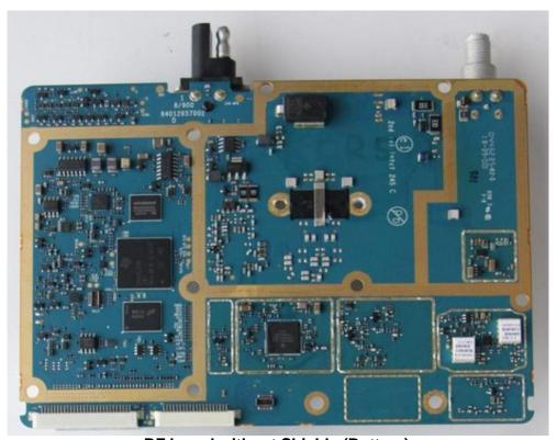
RF board without Shields (Bottom)
