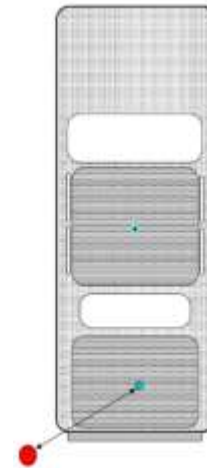
Test measurement setup for Bystander 45 degree (diagonal) trunk mount antenna
