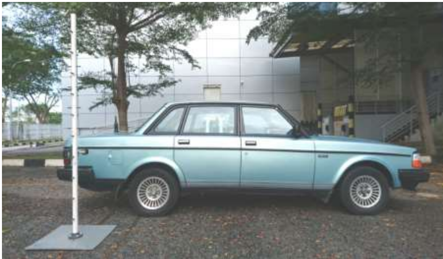
Test measurement setup for Bystander 90 degree (side) trunk mount antenna
