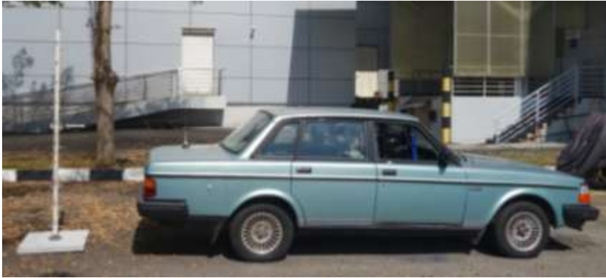
Test measurement setup for Bystander, trunk mount antenna behind vehicle
