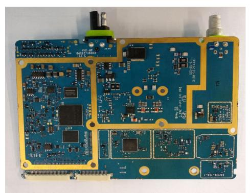
RF board without Shields (Bottom)
