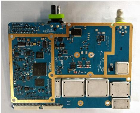
**RF board with Shields (Bottom)**
