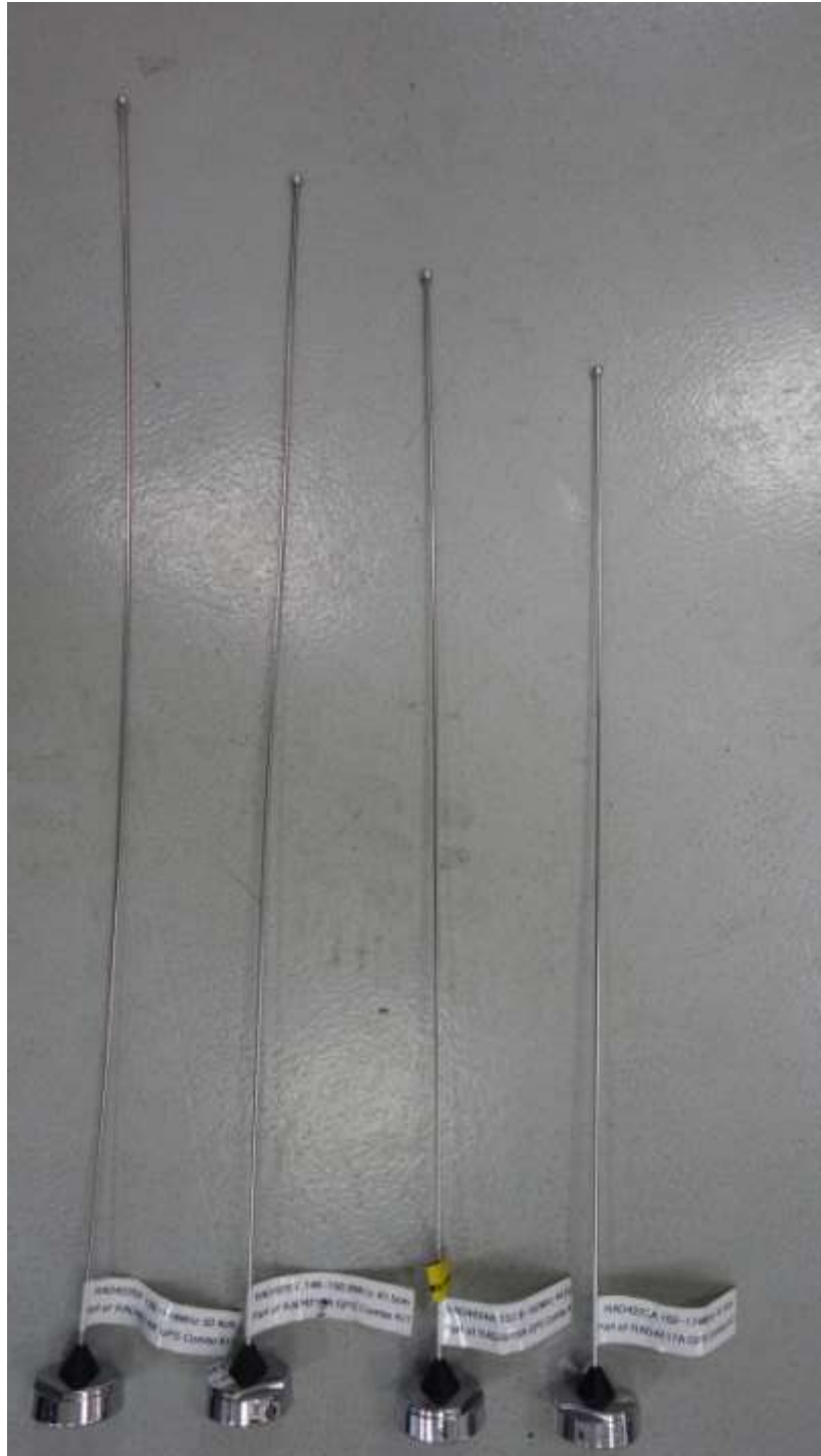
VHF Antenna kit numbers, from left to right RAD4226A, RAD4227A, RAD4224A, RAD4223A
