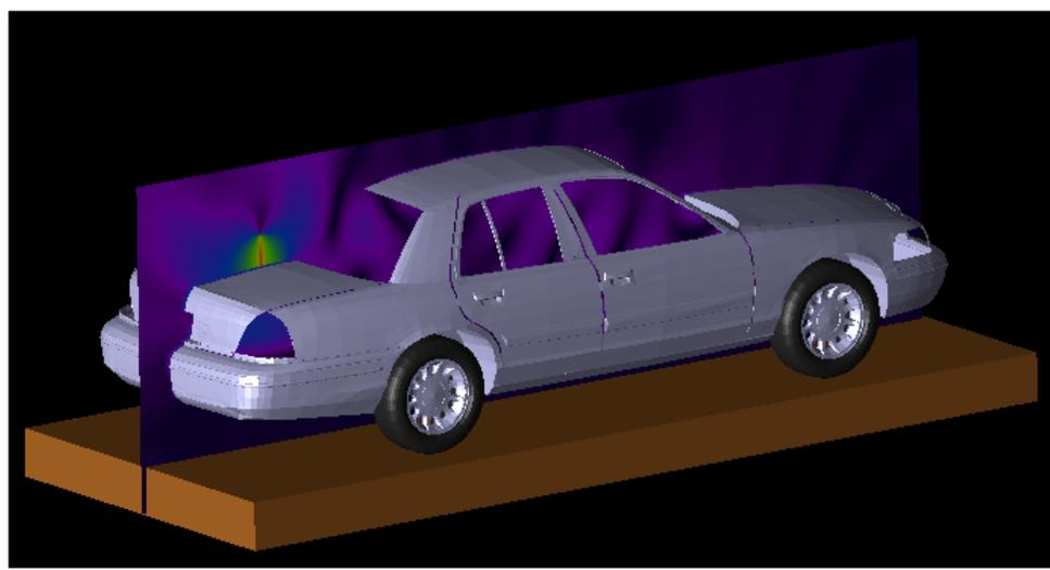
The equivalent power density ( $S$ ) is computed from the E-field and the H-field separately. The following table reports the E-field values computed by XFDTD™ at the six locations, and the corresponding power density.
