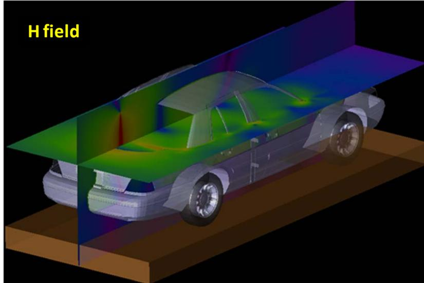
As done in the measurements, the equivalent power density ( $S$ ) is computed from the E-field, the H-field being much lower. The following table reports the E-field values computed by XFDTD™ at the three locations, and the corresponding power density.
