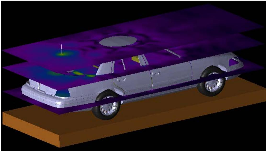
The equivalent power density (S) is computed from the E-field. The following table reports the E-field values computed by XFDTD™ at the three locations, and the corresponding power density.
