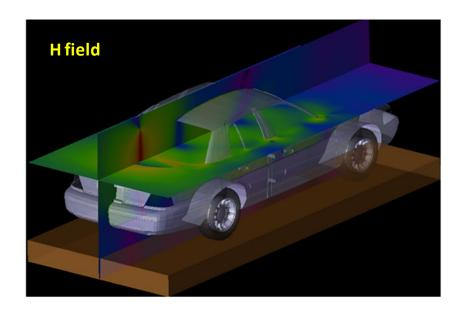
As done in the measurements, the equivalent power density (S) is computed from the E-field, the H-field being much lower. The following table reports the E-field values computed by XFDTD<sup>TM</sup> at the three locations, and the corresponding power density.
