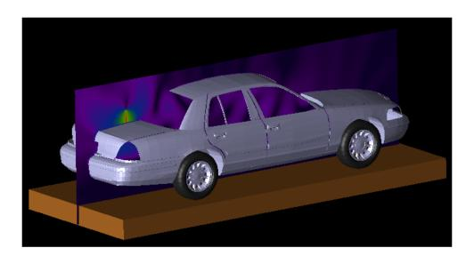
The equivalent power density (S) is computed from the E-field and the H-field separately. The following table reports the E-field values computed by XFDTD<sup>TM</sup> at the six locations, and the corresponding power density.
