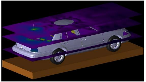
The equivalent power density (S) is computed from the E-field. The following table reports the E-field values computed by  $XFDTD^{TM}$  at the three locations, and the corresponding power density.
