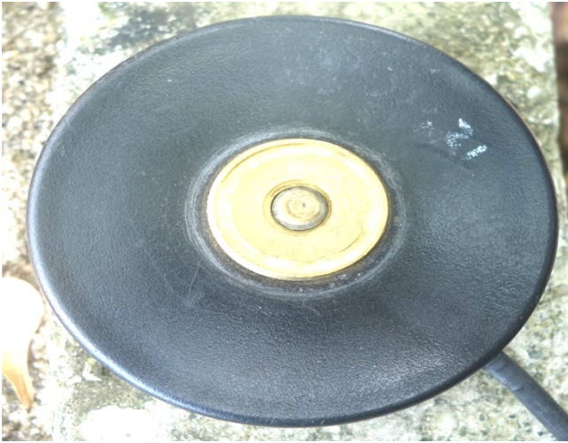
Magnetic mount base (top and side view)
