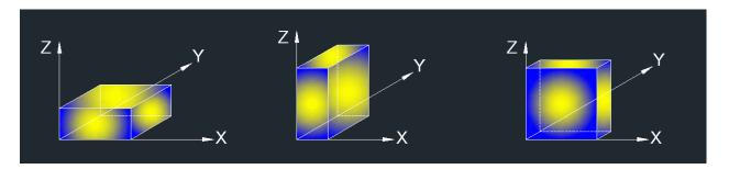
Note 1: For all radiated test, EUT in each of three orthogonal axis emissions have been tested, but only the worst case (X axis) data recorded in the report.
