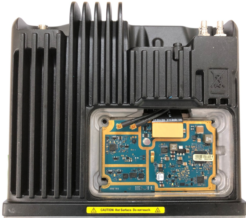
Exhibit 9F: Radio Assembly – Controller Board (Bottom View)
