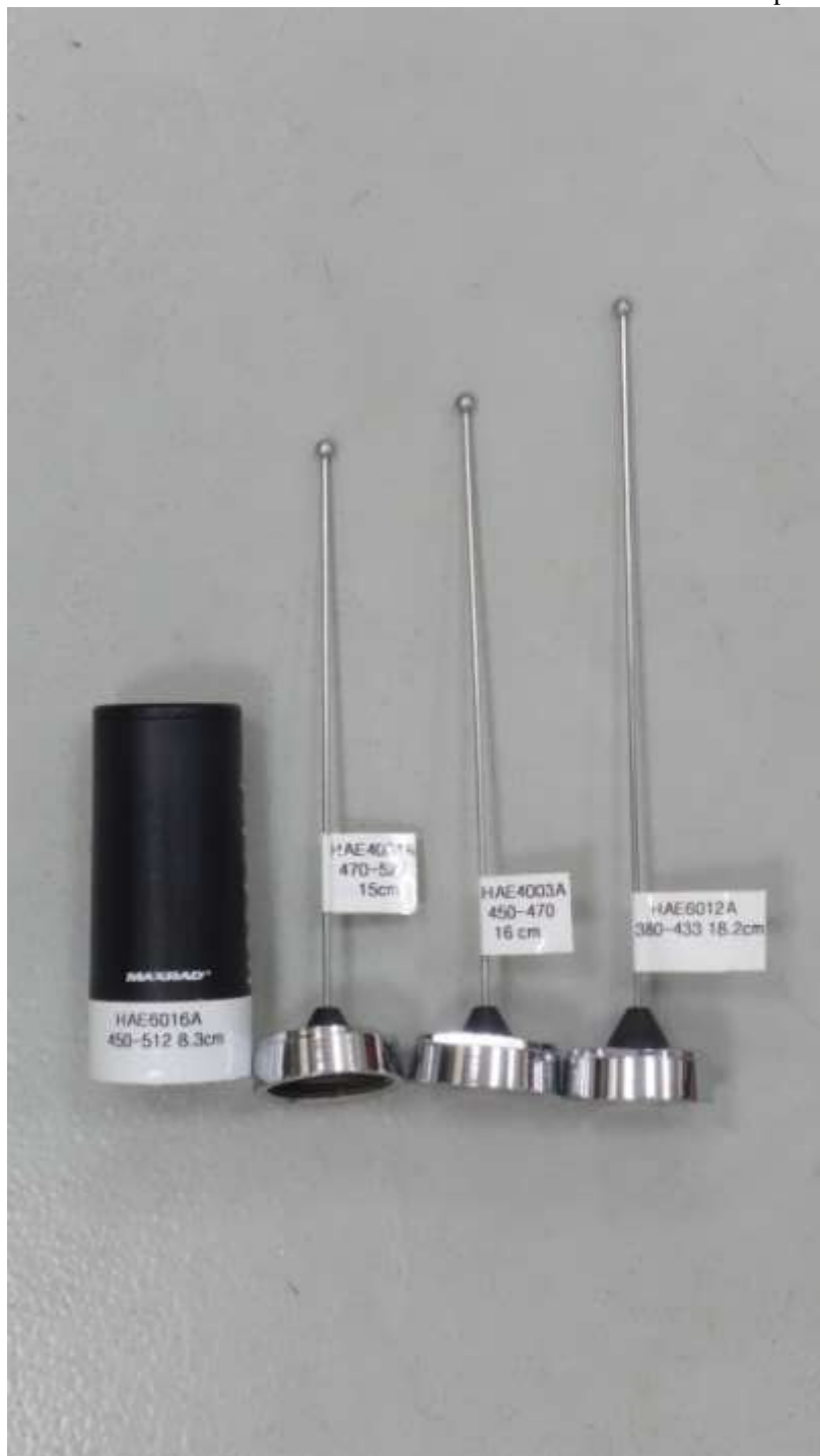
UHF Antenna kit numbers, from left to right; HAE6016A, HAE4004A, HAE4003A and HAE6012A
