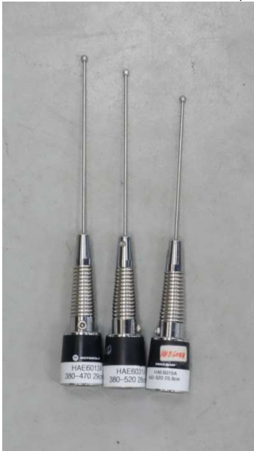
UHF Antenna kit numbers, from left to right; HAE6013A, HAE6031A and HAE6015A
