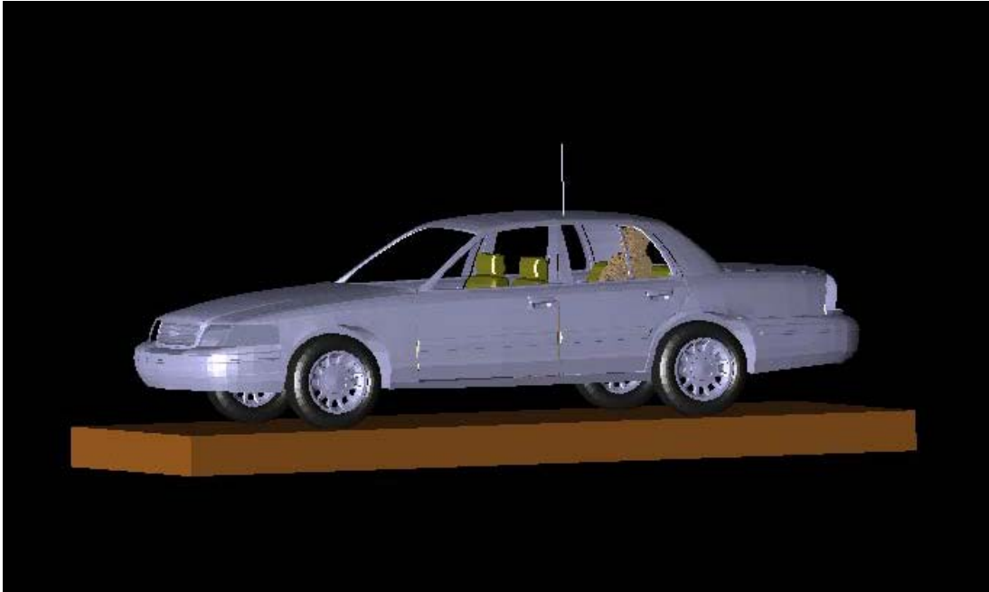
Figure 2: Passenger model exposed to a roof-mount antenna
