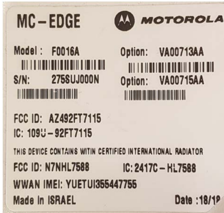
EXHIBIT 1B – FCC/IC Label for APX4000 7/800 for MC-EDGE with LTE options
