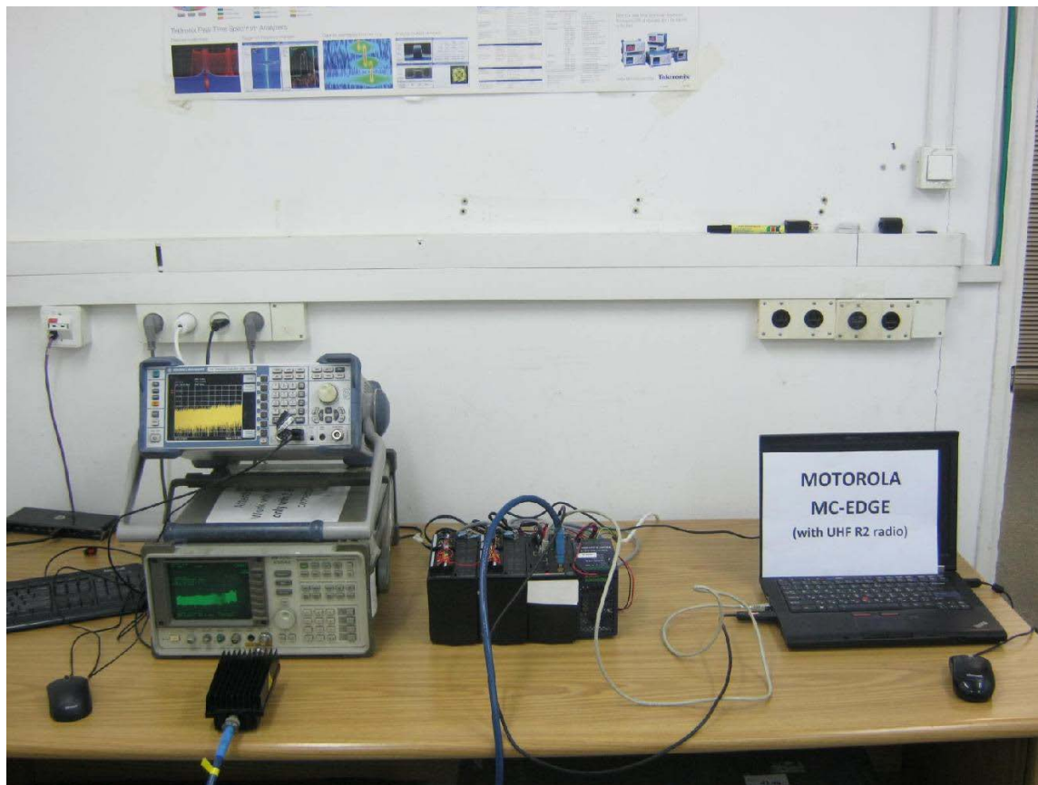
Figure 7 - 5 Conducted Emission Terminal Port Test
